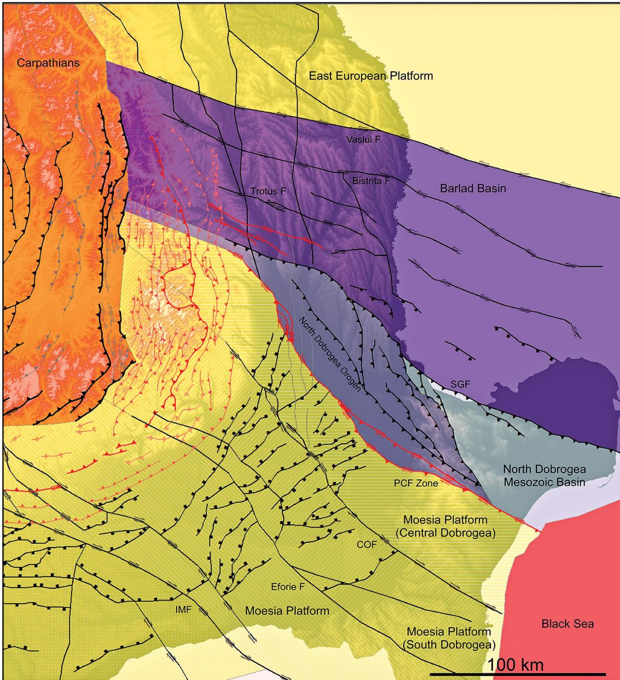
**Fig. 2.** Tectonic Map of Eastern Romania, compiled based on published material (Săndulescu, 1984; Getech unpublished study) (IMF – Intramosian Fault, COF – Capidava-Ovidiu Fault, PCF – Peceneaga-Camena Fault, SGF- Sf Gheorghe Fault).
