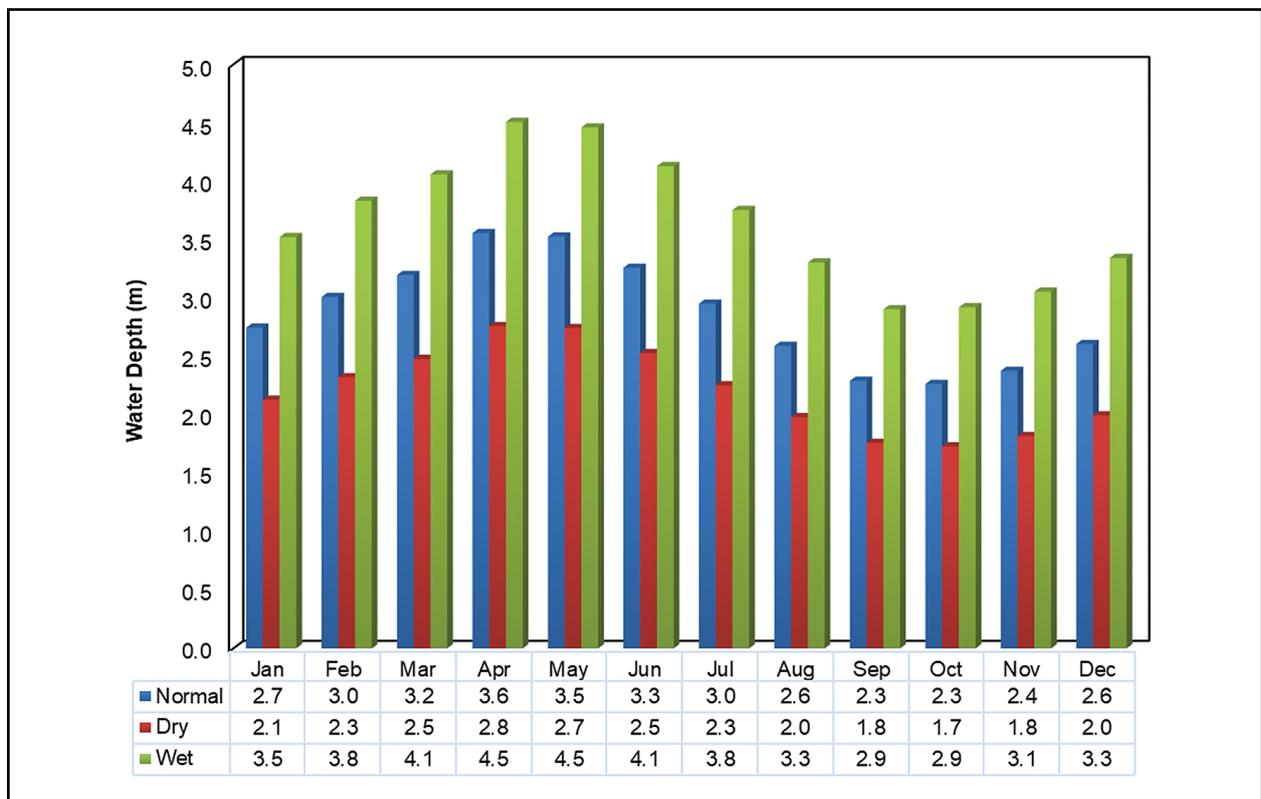
Fig 21. Water depths at the mid-cross section in dry, normal and wet flow years.
