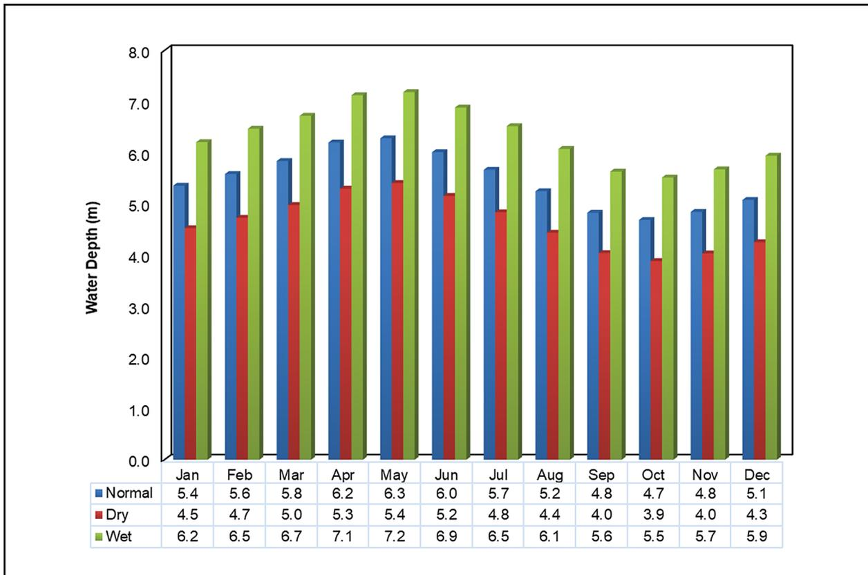
**Fig 22.** Water depths at the downstream cross-section in dry, normal and wet flow years.
