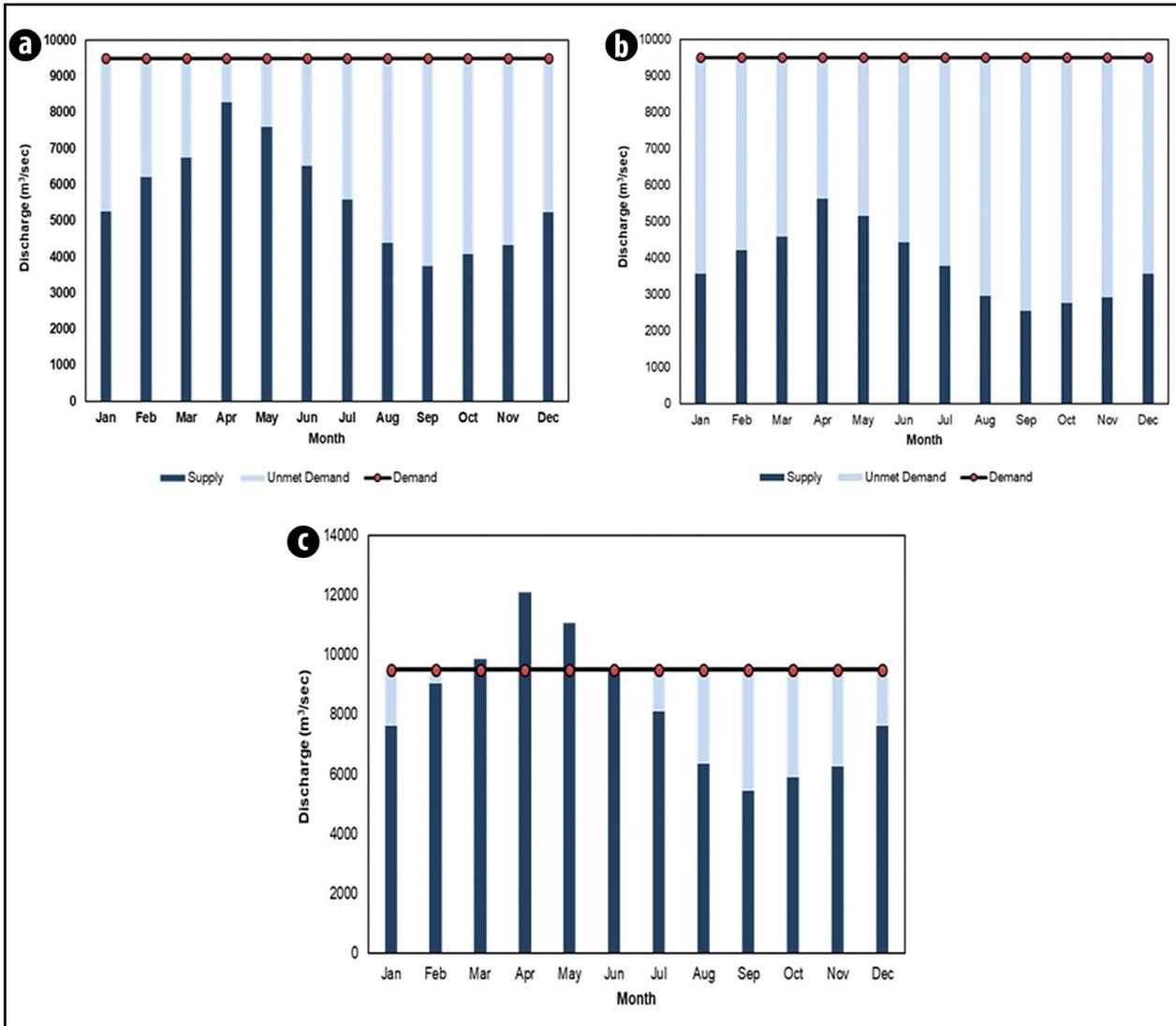
▲ Fig. 14. Water supply and demand for energy production in (a) Normal flow year, (b) Dry flow year, and (c) Wet flow year at IG II.
