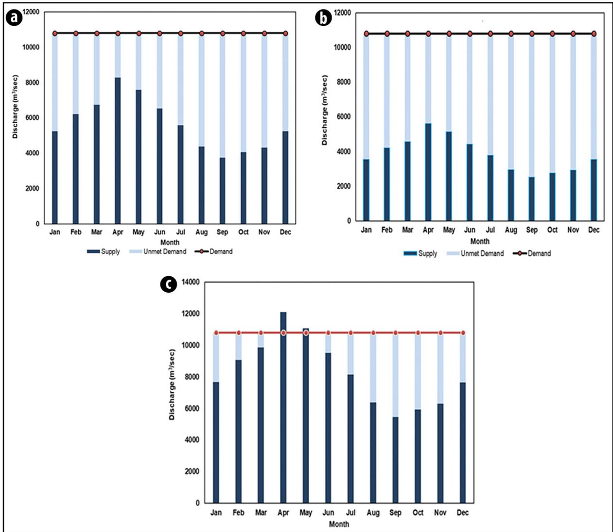
▲ Fig. 12. Water supply and demand for energy production in (a) Normal flow year, (b) Dry flow year, and (c) Wet flow year at IGI.
