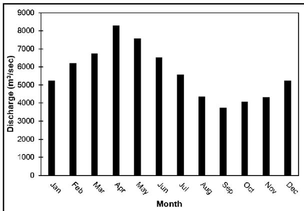
Fig. 10. flow boundary condition for the Danube river in HEC-RAS Model.
