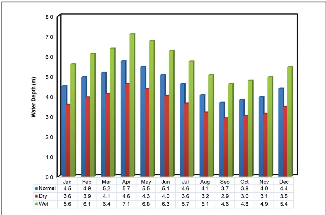
Fig. 20. Water depths at the upstream cross-section in dry, normal and wet flow years.
