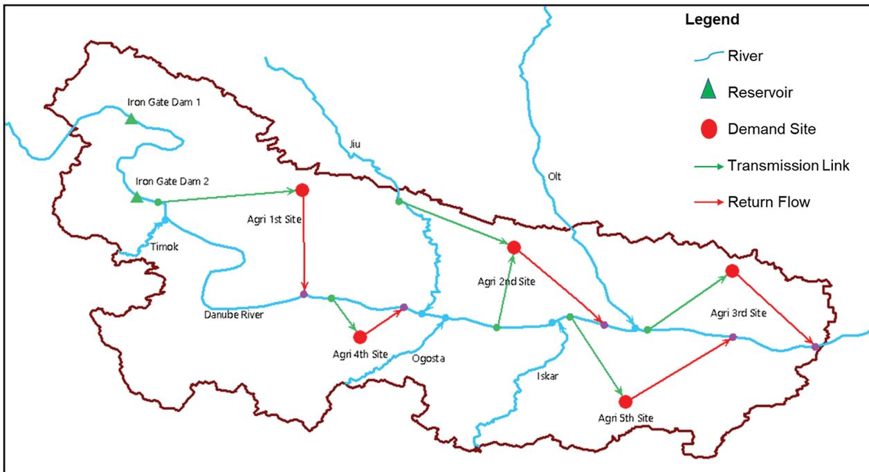
Fig. 8. Setup of the WEAP model, in which the points of agricultural demand are represented.
