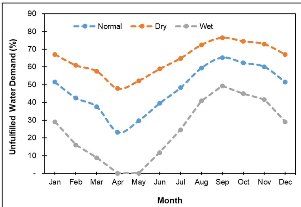
◀ Fig. 13. Unfulfilled water demand for energy production in dry, normal and wet year period at IGI.
