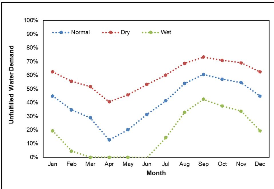
◀ Fig. 15. Unfulfilled water demand for energy production in dry, normal and wet year period at IG II.
