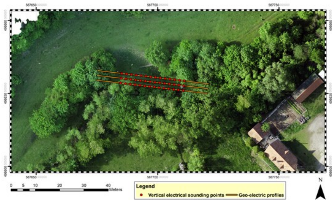
Fig. 2. Site plan of the three geoelectric profiles and the location of the VES points along them.
