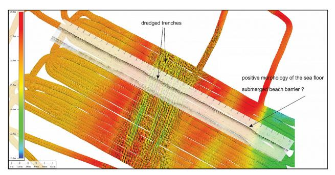
Fig. 8. Calibration of the seismo-acoustic facies on superimposed the images of DTM and SBP.
