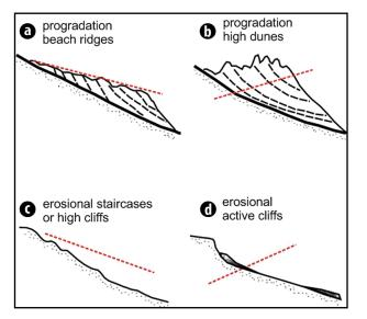
Fig. 3. Coastal development function of the relative sea level variation and availability of sediment a. falling sea level, high availability of sediment b. rising sea level, high availability of sediment c. falling sea level, scarce availability of sediment d. rising sea level, scarce availability of sediment (modified after Hansom, 2001).
