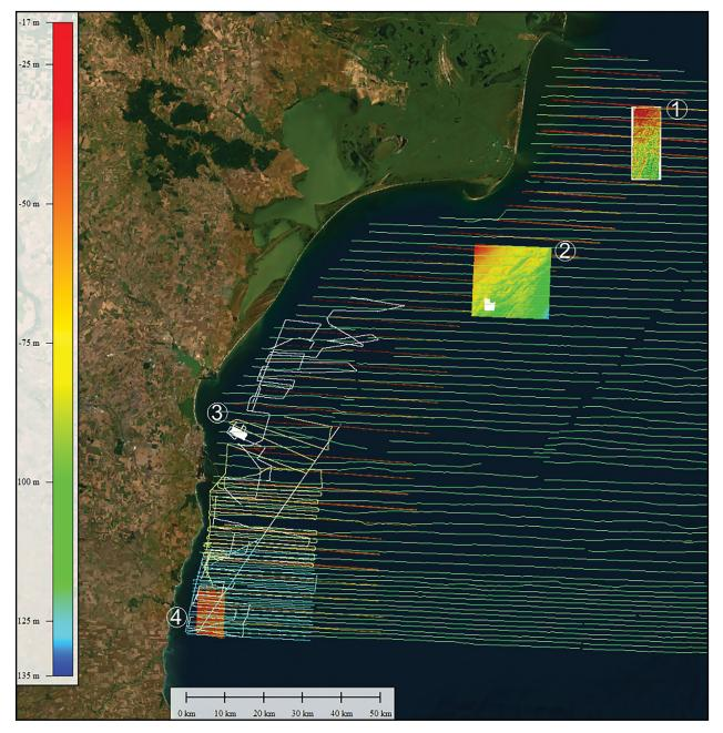
Fig. 4. Existing data in the area of interest (1, 2, 4 panels of DTM, 3 panel of DTM, SSS, and SBP): green lines – SBP 3.5 kHz; orange lines – MBES; yellow – MBES+SBP (chirp 2-12 kHz); cyan – MBMES + SBP (chirp 2-12 kHz); white – MBES+SBP (chirp 2-12 kHz).
