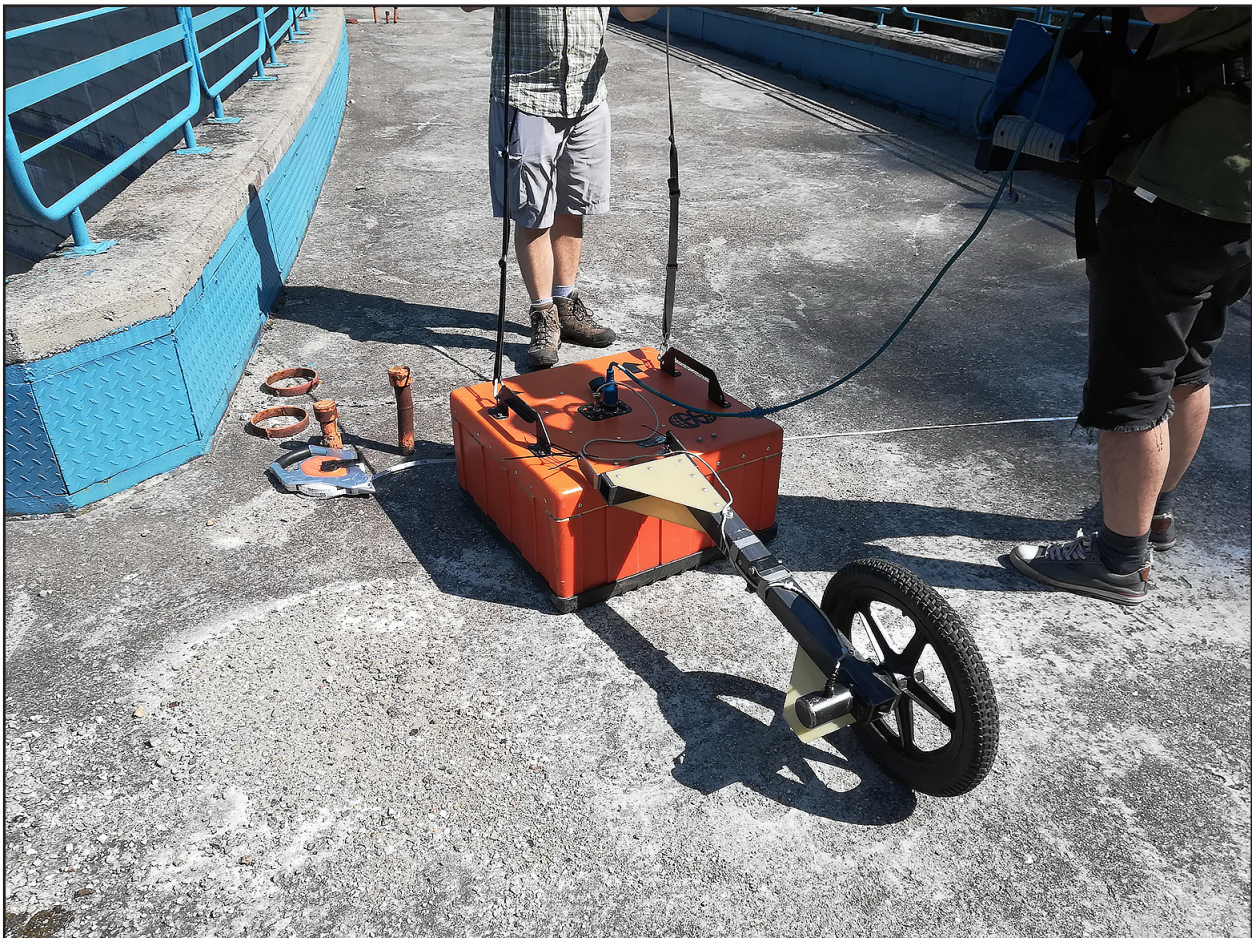
Fig. 3. The GSSI SIR-3000 GPR system used to collect the GPR data, consisting of a 200 MHz antenna, a wheel and a console.
