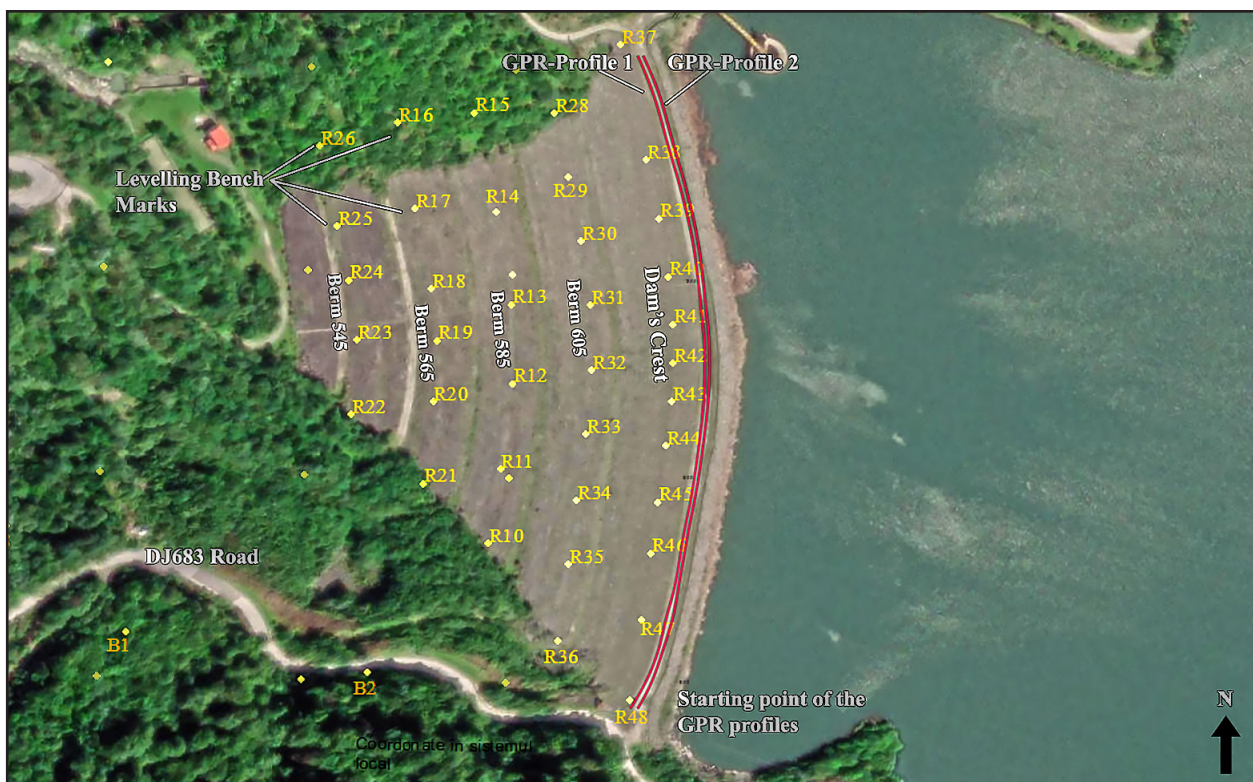
Fig. 2. Overview of the Levelling Network, with visible bench marks on different berms. The position of the GPR profiles on the dam's crest is also shown.
