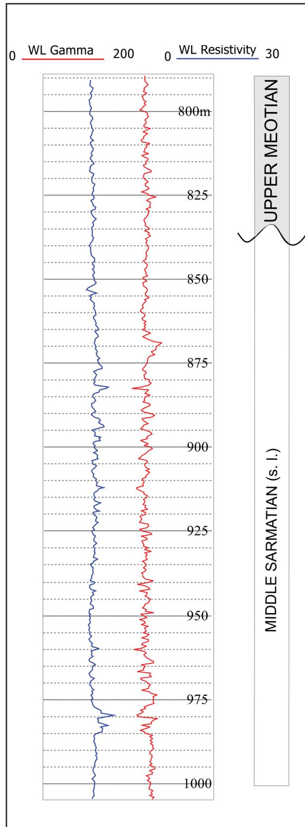
**Fig. 5** Well logs of the Middle Sarmatian (s.l.) and Upper Meotian deposits crossed by the Băleni-1 borehole
