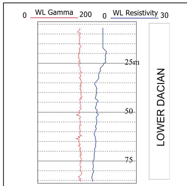
Fig. 3 Well logs of the Lower Dacian deposits crossed by the Baleni-1 borehole
