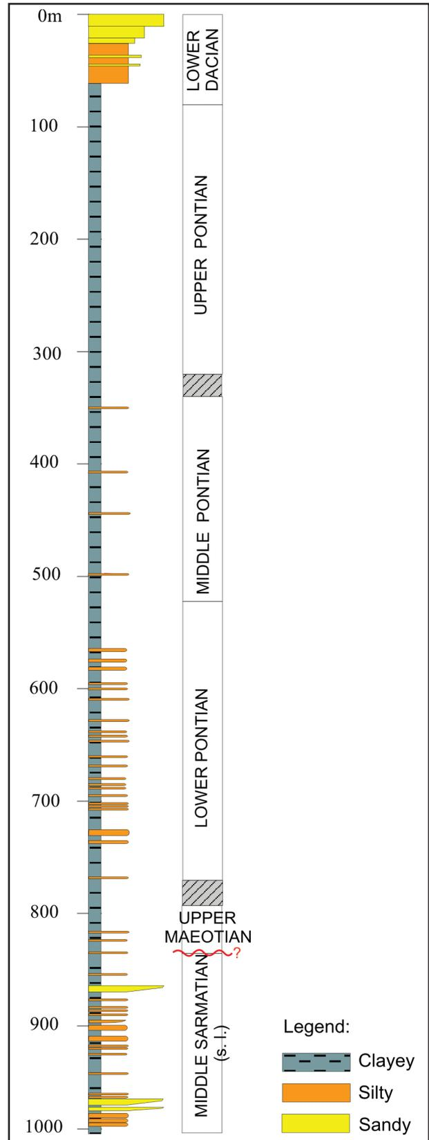
**Fig. 7** Estimated lithology of the Sarmatian (*s.l.*) – Dacian deposits drilled at the borehole location Baleni-1. The sedimentary column is based on cutting observation and well logs shape
