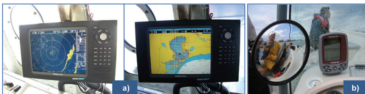
Fig. 3 Equipments used for location of the sampling stations and for water depth and temperature measurements. a) "Simrad" Radar-GPS-Echo-sounder equipment; b) "Eagle-Cuda-168" echosounder.
