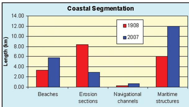
Fig. 6 Landforms vs. port/coast-protection structures
