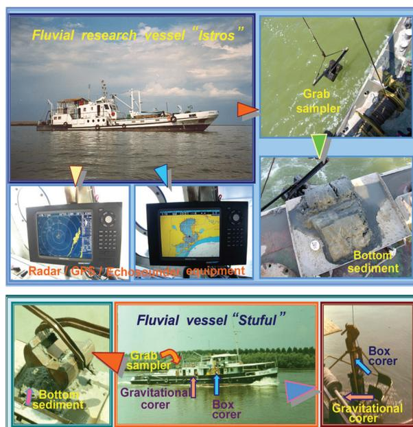
Fig. 2 Research vessels and sampling equipment.
