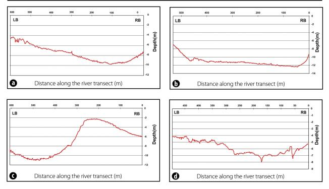
Fig. 6. Cross sections on the Danube River (LB – Left bank; RB – Right bank). (a) Km 557 Upstream Zimnicea; (b) Km 789 Downstream Calafat; (c) Km 551 Downstream Zimnicea; (d) Km 687 Kozlodui
