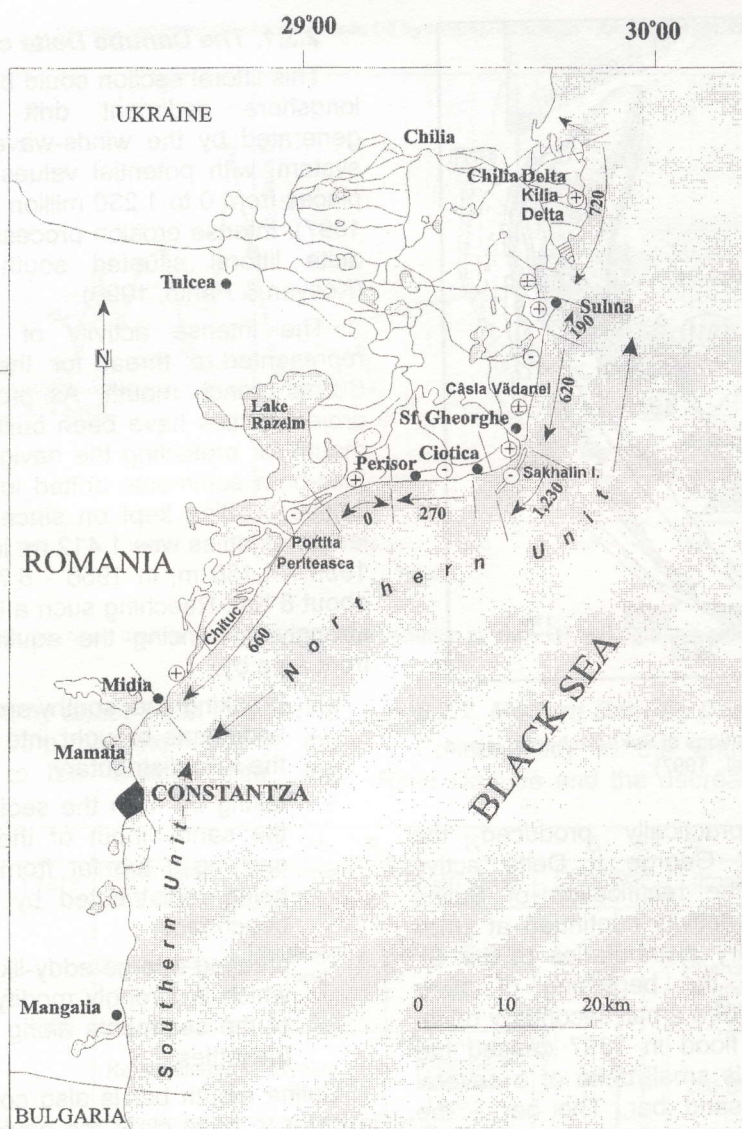
Fig. 9 Romanian Black Sea coast and the longshore sediment transport model for the Danube Delta coast. Transport rates in thousands of cubic meters per year. Circled + and - represent advancing and retreating sections respectively (after Giosan et al., 1997)
